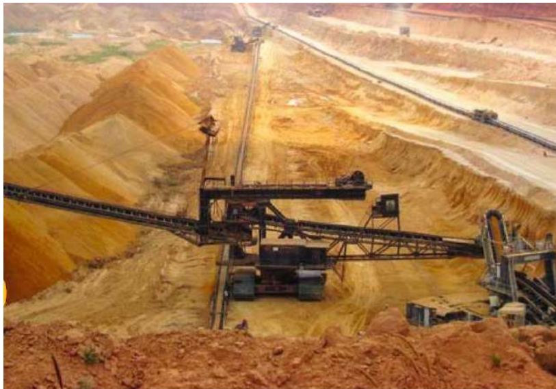
Open-pit mining of phosphate rock in Togo. Most of the world's phosphate rock is extracted from open pits, as shown here, or from large-scale mines equipped with drag lines or shovel/excavator systems. Credit: Alexandra Pugachevsky
