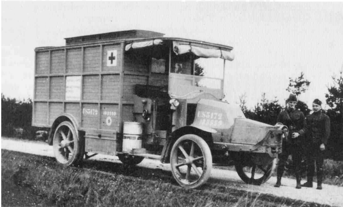
Renault truck outfitted with mobile x-ray equipment
