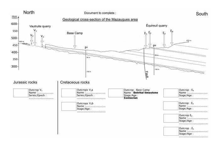
Let us begin your investigation by looking at the piezometers (P1 at BaseCamp, and P2 at Equireuil quarry). Read the water level in each piezometer well.
